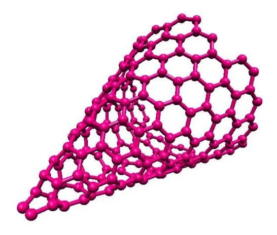
Figure 2. The structure of carbon nanocone
