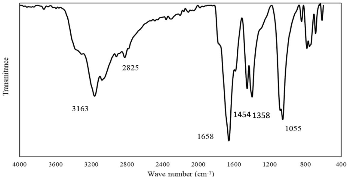
**Figure 1.** FTIR spectrum of synthesized oleamide
