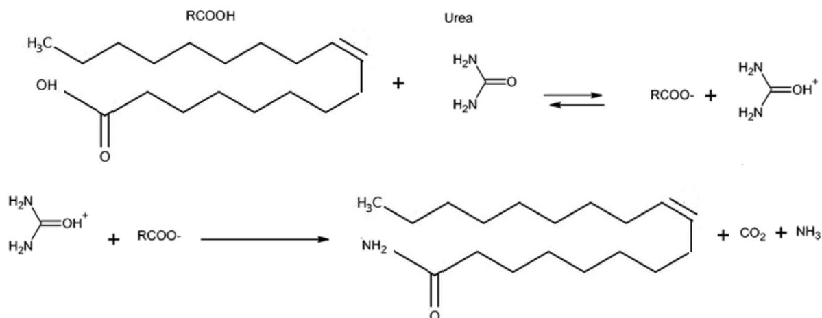
Figure 6. Proposed mechanism of oleamide synthesis
