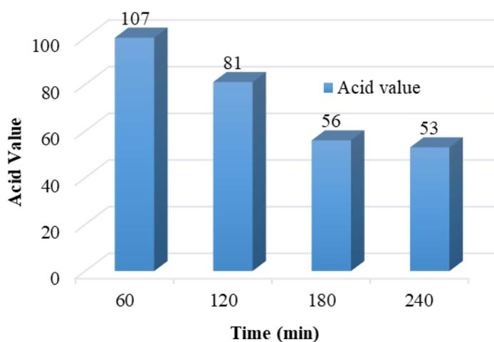
**Figure 4.** The effect of reaction time on acid value at 200 °C and oleic acid: urea molar ratio of 1:4 in the presence of 1 wt%  $\text{AlCl}_3$
