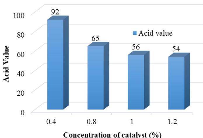
**Figure 5.** The effect of catalyst concentration on acid value at 200 °C, reaction time of 180 min and oleic acid / urea molar ratio of 1:4
