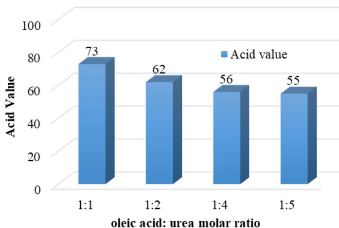
**Figure 2.** The effect of oleic acid: urea molar ratio on acid value at 200 °C and 180 min reaction time in the presence of 1 wt%  $\text{AlCl}_3$
