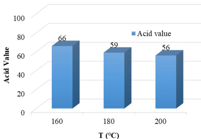
**Figure 3.** The effect of temperature on acid value at oleic acid: urea molar ratio of 1:4 and 180 min reaction time in the presence of 1 wt%  $\text{AlCl}_3$
