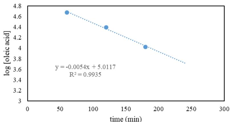
**Figure 7.** The plot of log[oleic acid] versus time
