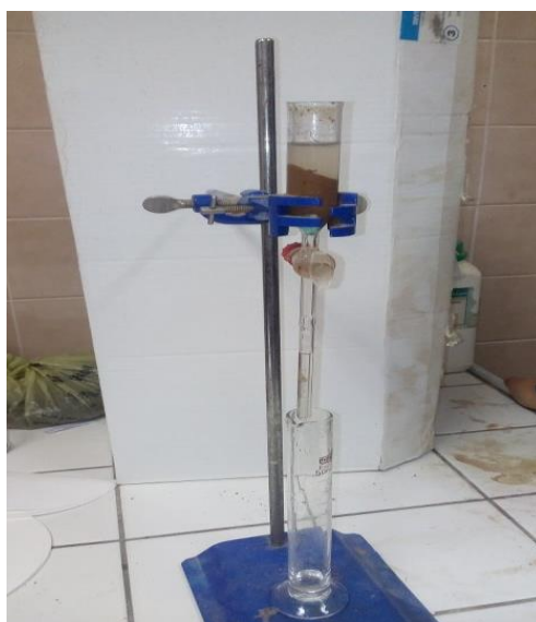
Fig. 1: Determination of soil permeability using a glass column
