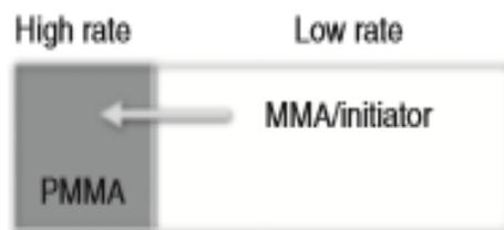
**Figure 4:** Schematic of isothermal polymerization.
