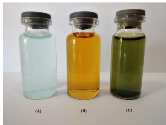
Figure 2. Synthesis of CuNPs using Pomegranate Peel extract: (a) Test tube containing 1 mM Cu (NO 3 ) 2 H 2 O. (b) Pomegranate Peel extract (c) CuNPs after 2hrs
