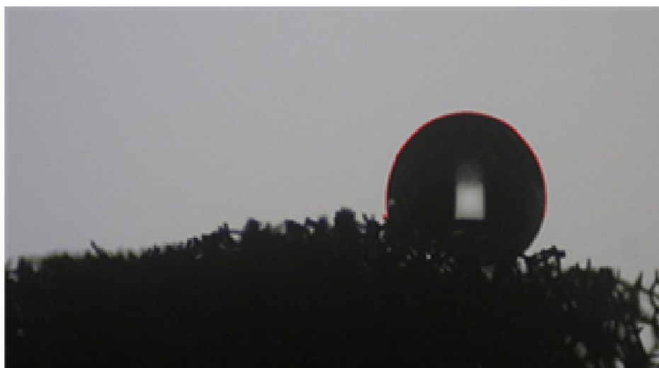
Figure 1. Optical image of a water droplet on NiFe 2 O 4 /PU sponge
