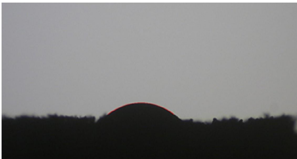
Figure 2. Optical image of an oil droplet on \text{NiFe}_2\text{O}_4/\text{PU} sponge
