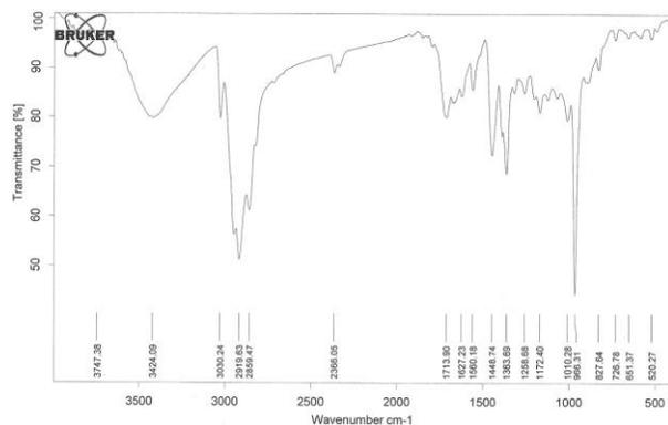
Figure 2. FT-IR spectrum of  $\beta$ -carotene
