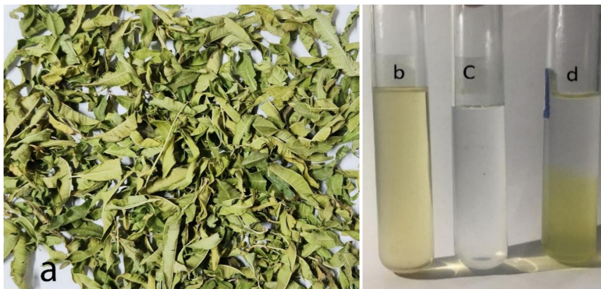
Figure 1 a) Aloysia Citrodora plant b) Aloysia Citrodora water extract c) Zinc acetate Solution d) biosynthesized ZnO NPs using Aloysia Citrodora water extract
