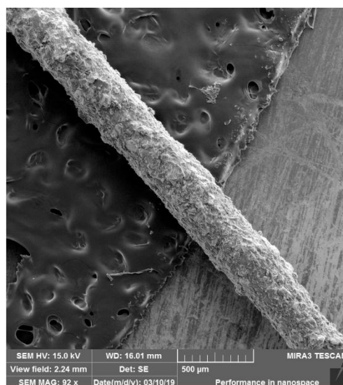
Figur.2. The morphology of the surface structure of the prepared fiber
