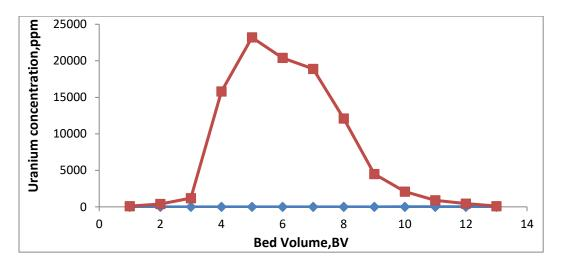
**Figure 7.** Elution curve of uranium loaded macroporous D201 resin using 1.0 M sodium chloride acidified by 0.1M H<sub>2</sub>SO<sub>4</sub>
