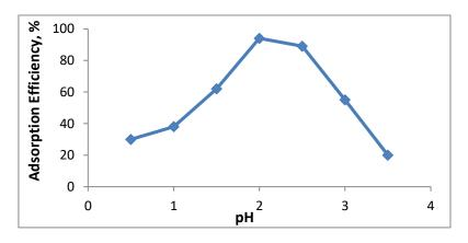
**Figure 1.** Effect of pH on uranium adsorption efficiency using macroporous D201 resin (Conc. 500 ppm at 25 °C)
