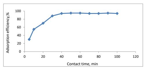
Figure 2. Effect of contact time upon the uranium adsorption efficiency on D201 resin
