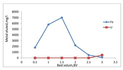
Figure 9. Selective iron elution from the loaded D201resin column using SMBS
