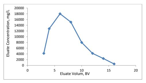
**Figure 10.** Elution of uranium loaded upon macroporous D201 resin after Fe eluted Conversion (re-usability)
