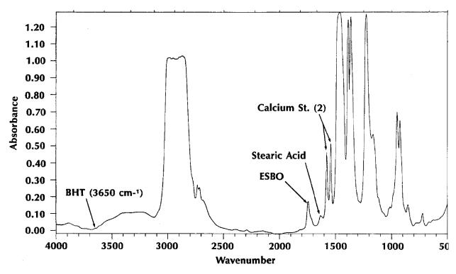
**Figure 1.** Example of an FTIR Spectrum for butyl rubber (from ref 6).
