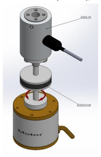
**Figure 5.** Schematic diagram of the dynamic rheometer (GTM-GmbH)
