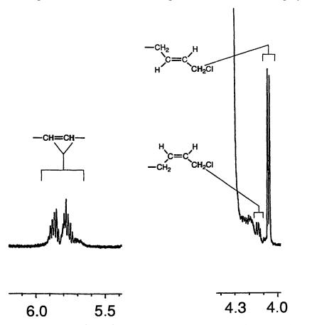
Figure 2. 500-MHz 1H NMR spectra of a suspension PVC (from ref 8).
