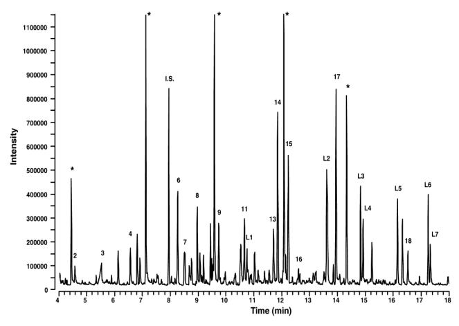
**Figure 7.** GC-MS chromatograms after 1,200 hours of aging of polyamide 6,6 at 100 oC. Peaks 1–18: low molecular weight degradation products evolved (including cyclic imides, pyridine derivatives, chain fragments, and cyclopentanones). L1–L7: alkanes and alkenes from a lubricant added to the polymer. S.I. D internal standard (from ref 12).
