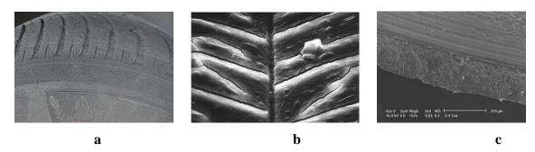
**Figure 3.** Cracks on tire (a), Polypropylene molded part (solvent induced stress cracking at seam.) 750× (b), Close-up of ozone crack using ESEM (c)
