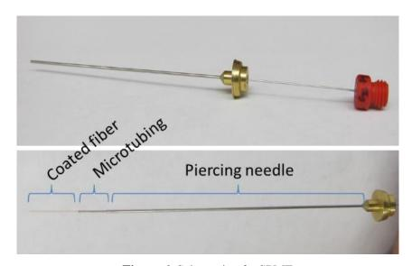
Figure 6. Schematic of a SPME
