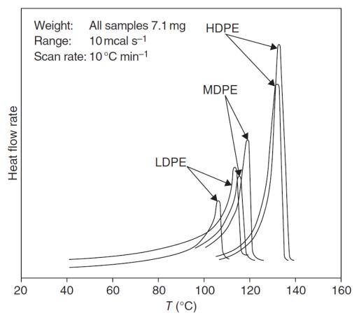
**Figure 4.** DSC of various polyethylenes (from ref 10)
